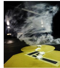
The KP buildings subjected to WindEEE tornado
