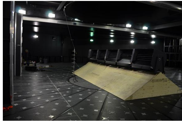
The RB2 model on the roof in the WindEEE test chamber
